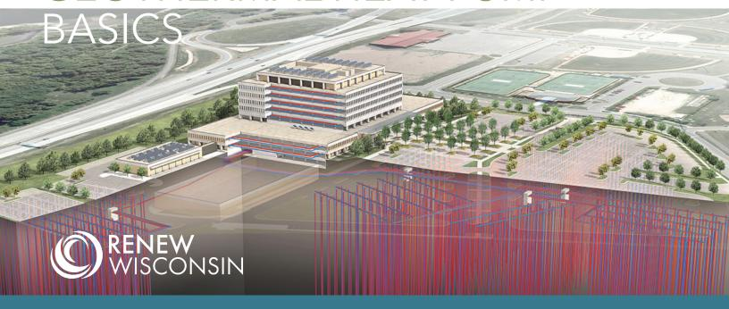
Geothermal energy is a renewable, all-electric technology that uses heat from the earth to heat and cool buildings. "Ground source heat pumps" is another name for this technology.
