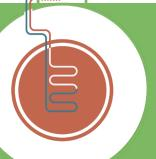
The **GROUND LOOP EXCHANGER** is a system of underground pipes circulating a liquid that *exchanges* heat with the earth.
